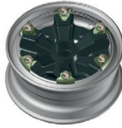
DEMOUNTABLE WHEELS, 15° DROP CENTRE FOR TUBELESS TYRES
