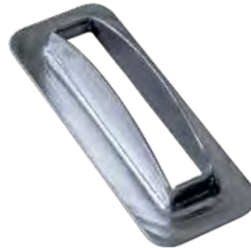
Rectangular slotted eyelet Inner dimensions 38 × 8 mm, height 10.3 mm, zinc plated steel. 320133039
