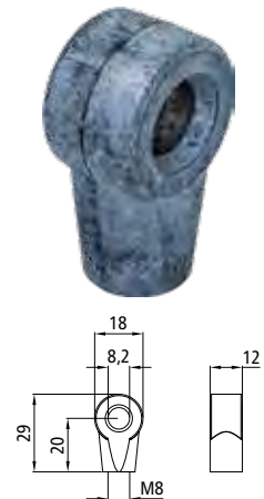
Round-eye connectors With female thread M8, zinc plated steel, weight 0.02 kg. 215141734
